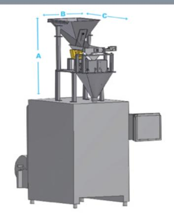
SPECIFICATIONS: Height (A) Width (B) Depth (C) iQ-Shuttle over bagger: 48 inches 25 inches 42 inches iQ-Shuttle on stand: 90 inches 42 inches 48 inches
